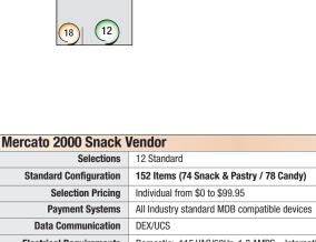
**Electrical Requirements** Domestic: 115 VAC/60Hz, 1.2 AMPS International: 230 VAC/50Hz, 0.6 AMPS 33-1/2" (85 cm) Dimensions 72"(183 cm) Width 21" (53.3 cm) Depth Height Net Weight 350 lbs. (158.8 kg) **Standard Features** GVC1 Controller with 4 Digit LED Display, Braille Keypad Options inDEX Tool (Pricing Only), 4" Legs, Custom Colors, Custom Graphics
